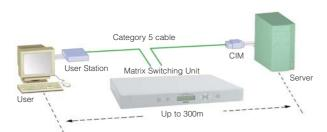
• **Category 5 UTP cable connections**, enabling extended distances between users and servers up to 300m apart, replacing costly, hard-to manage, distance-limited coaxial cable;
